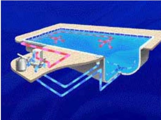
The circulation system has a dramatic affect on the health of a pool. When water is in motion, it's harder for bacteria and algae to find a surface on which to grow and the chemicals are more thoroughly distributed. In addition, as the water passes through the filter, debris is captured for easy removal.
